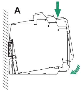
A. Snap metal lock onto mounting rail, then rotate the devices, as figure A, press down the devices onto mounting rail.
