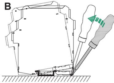
B. Pry the metal lock off the rail with screwdriver as arrow shown, pull downward the springs, and rotate the devices.
